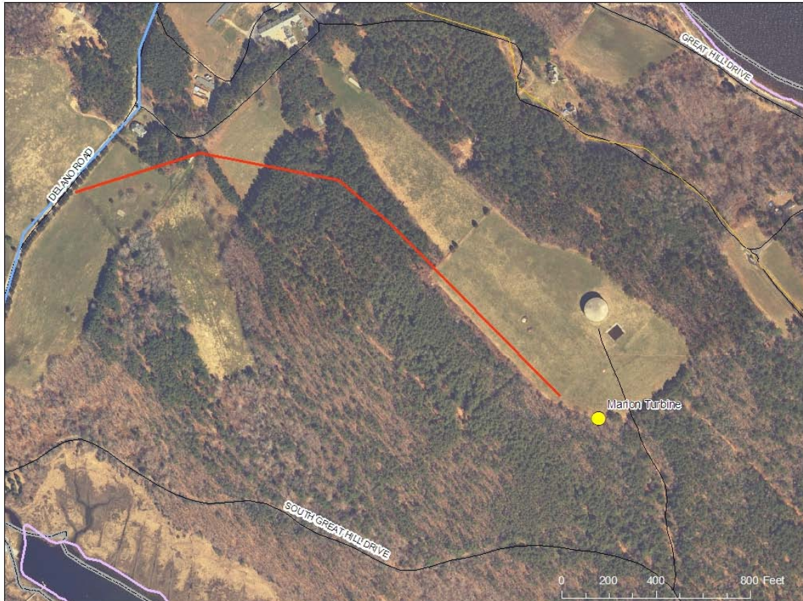
Figure 5-6. Potential Turbine Access Road.
